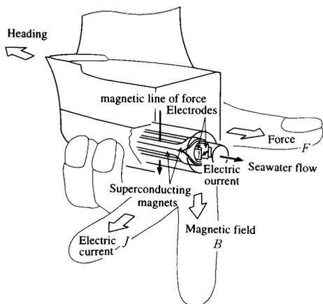
Fig. 1 Principle of MHD Propulsion Ship
