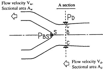
**Fig. 12 Pressure Measuring Positions in 6 Branch Pipes**
