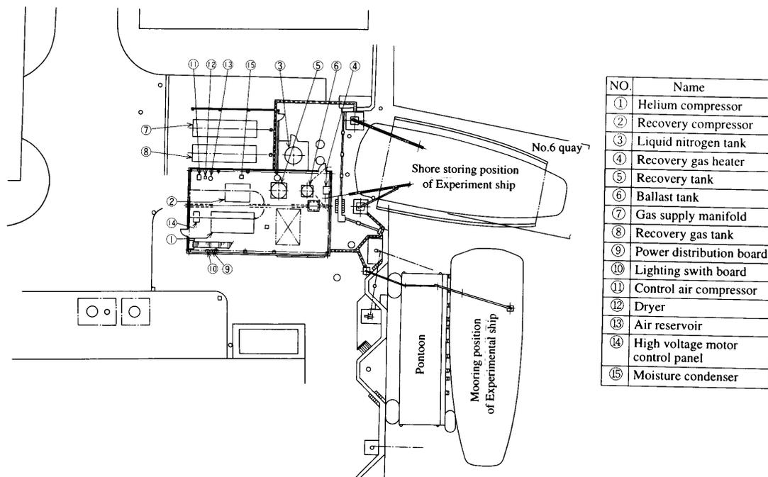
**Fig. 6 General Arrangement of Shore Support Base**
