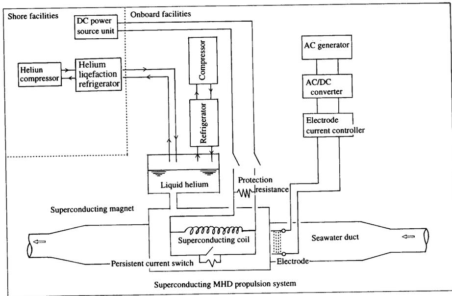
Fig. 3 Outline Diagram of Propulsion System "YAMATO 1"
