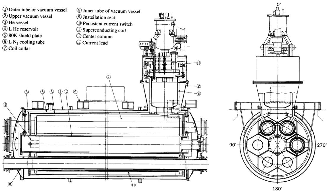
**Fig. 4 General Assembly of 6-linked Ring Magnet**
